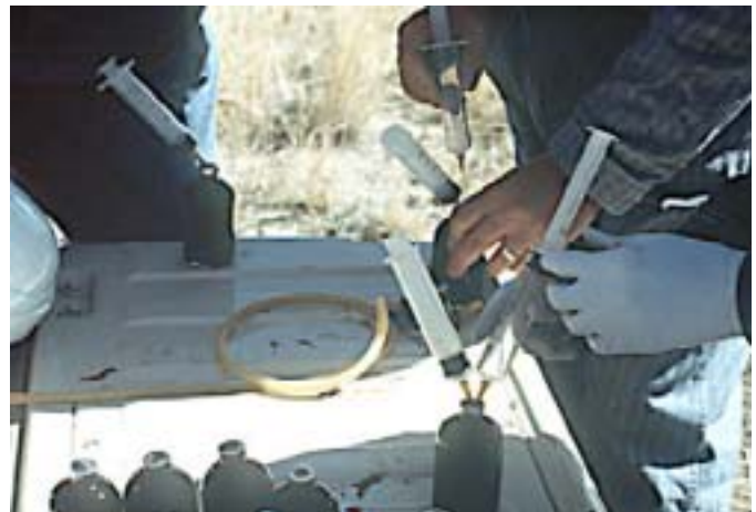
Figure 8. Introducing an inert gas (N 2 ) headspace over well-head samples to prevent oxidation and preserve samples for laboratory analysis.
