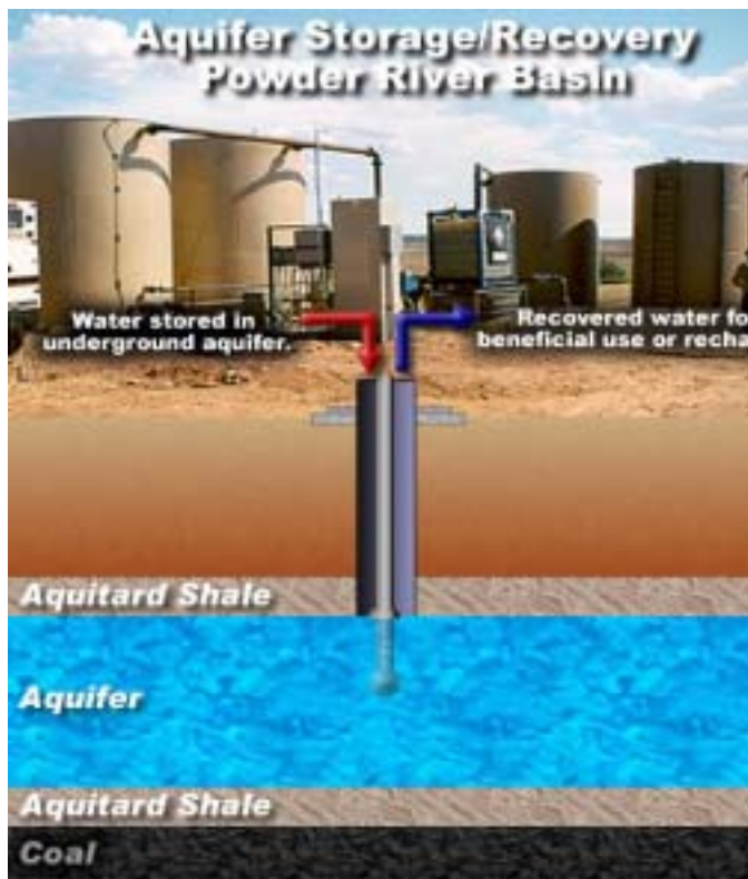
Figure 17. Well schematic of aquifer storage and recovery.
