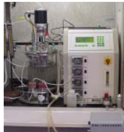
Figure 9. Bioreactor operating on a gas feed of hydrogen sulfide. The inoculum is a microbial consortium of nitrate reducing sulfide oxidizing bacteria.
