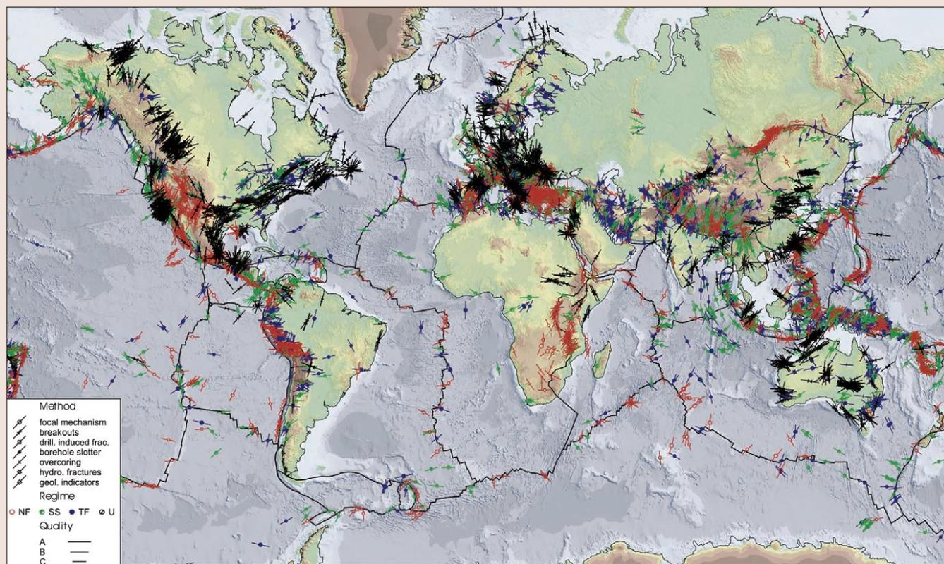
**Figure 1.** The World Stress Map consisting of more than 10 500 A-C quality stress indicators from a variety of stress measurement techniques. NF = normal faulting stress regime (red). SS = strike-slip (green). TF = thrust fault (blue). U = undefined (black). See legend for more details on symbols. All data and maps are freely available on the WSM Web site: [www.world-stress-map.org](http://www.world-stress-map.org).
