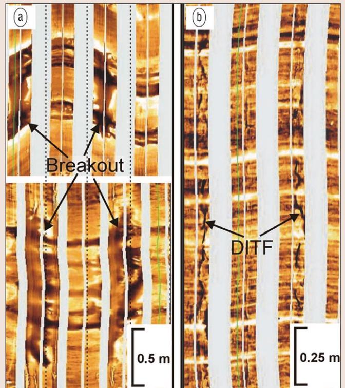
**Figure 2.** Examples of (a) borehole breakouts and (b) drilling-induced tensile fractures (DITF) observed on a resistivity image log (Formation Micro Imager). Borehole breakouts are poorly resolved, conductive zones separated by 180° and form perpendicular to the maximum horizontal stress orientation. DITFs are narrow conductive fractures that are typically subparallel to the borehole axis and separated by 180°. DITFs form parallel to the maximum horizontal stress orientation.
