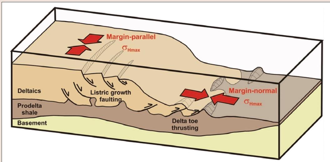
**Figure 5.** Schematic relationship between present-day stress and structures in passive-margin Tertiary deltas (adapted from Yassir and Zerwer, 1997). The convex upward shape of the clastic wedge promotes gravity-driven extension toward the delta toe, resulting in margin-parallel maximum horizontal stress orientations on the shelf and margin-normal thrusting in the delta toe.
