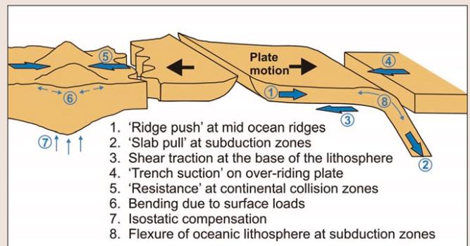
**Figure 3.** Forces controlling the present-day tectonic stress field at the plate-scale (large blue arrows) and broad regional scales (small blue arrows). (Adapted from Zoback et al., 1989)
