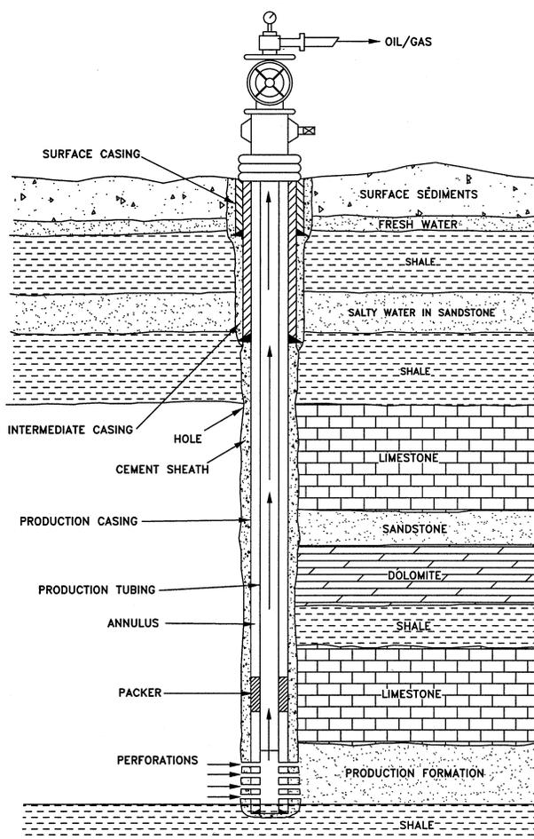
**Figure 3. Typical well construction.**
