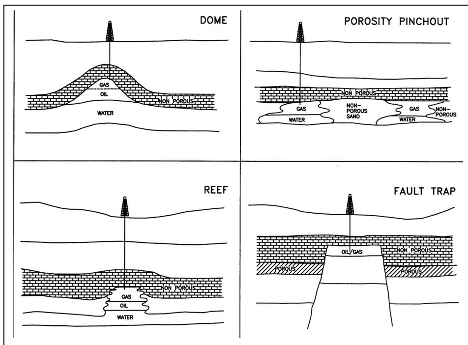
**Figure 2. Common types of traps in which oil and gas are found in southern Ontario.**
