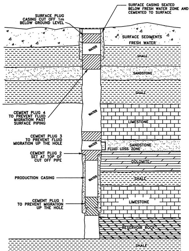
Figure 4. Typical plugged well.
